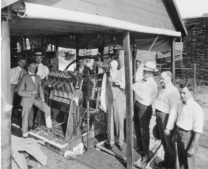
Packard and Lincoln personnel review the first running prototype of the Liberty engine at the Detroit Packard plant on July 28, 1917. The prototype was an eight-cylinder configuration, but most of the Liberty production was the twelve-cylinder version. Wilfred Leland is to the left of the engine. Henry Leland is immediately in front of the engine, discussing it with Alvan Macauley, president of Packard. Photo courtesy of NAHC, Detroit Public Library.
