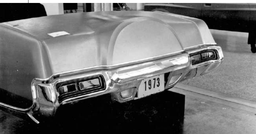
■ Impact bumpers were required on the rear of the Mark IV beginning in 1973. Designers thought they ruined the looks of the cars they designed.
