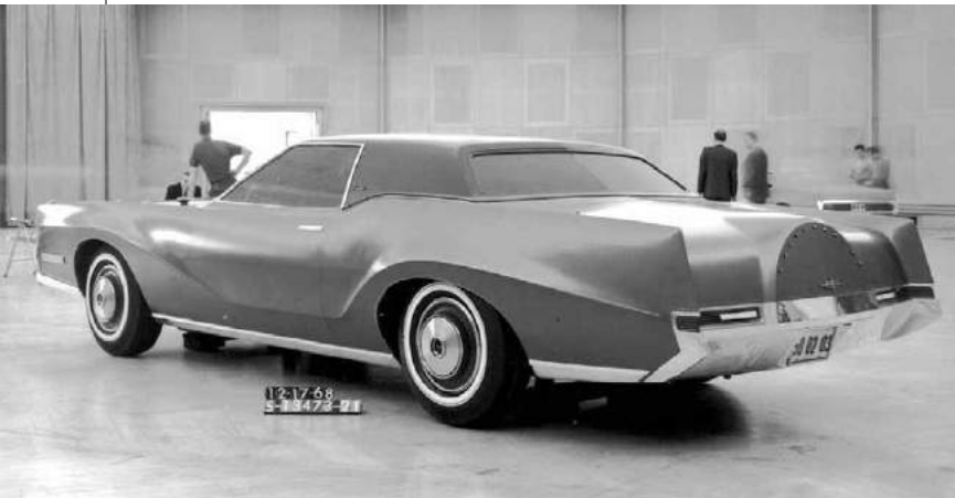
■ The final rendition of the Sherer/Perry alternate Mark IV proposal had wheel arches that flowed in a continuous line along the entire bodyside of the car.
