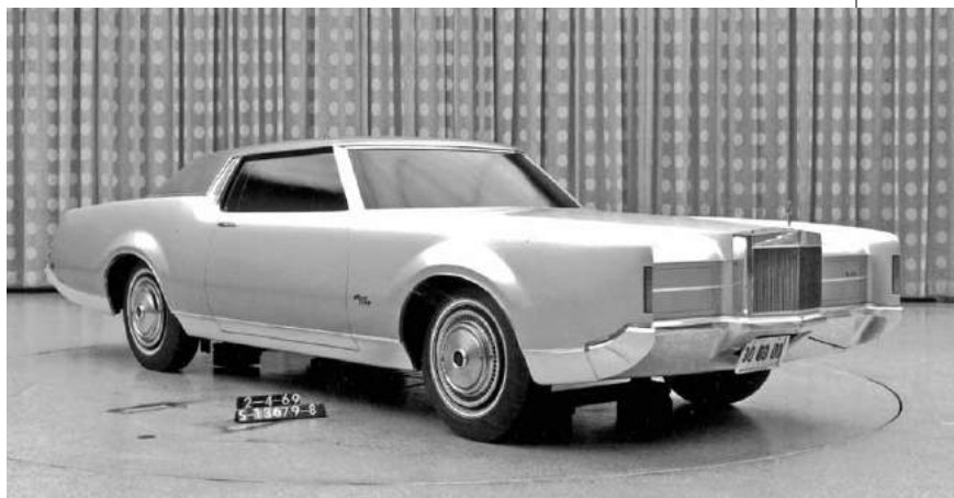
■ Designer Dean Beck originally wanted a well-defined centerline on the top of the grille shell of the Mark IV, as shown in this photo.
