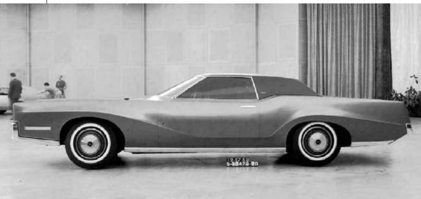
■ The highly accented wheel arches were later incorporated on an early proposal for the Lincoln Town Car. They were removed when an aftermarket contractor pointed out that they would make it more difficult to stretch the car when making it into a limousine.
