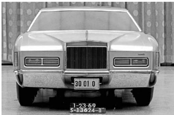
■ The original Mark IV proposal designed by Dahlberg's group included rectangular headlamps, as shown in this photo.
