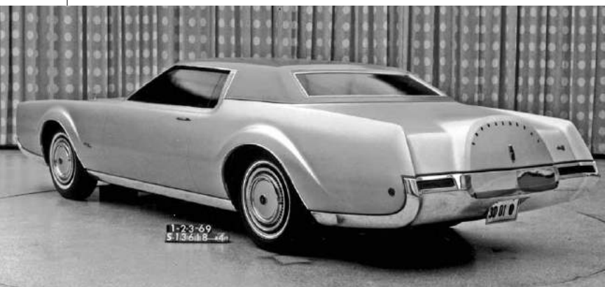
■ Arches are incorporated above the wheelwells on this version of Dahlberg's Mark IV proposal. Knudsen quickly ordered them removed.
