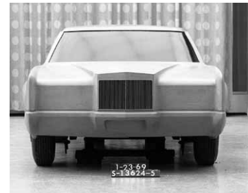
■ Left: This is the first photo found of a smaller Mark V proposal. It is dated 1-23-69. This car does not appear to have the same windshield slope as Marks traditionally have. According to retired Ford designer Dick Nesbitt, this car is almost identical in shape to the Torino/Montego-based Mark V in the Lincoln studio several years later. Center: From the back, the same car looks pinched. Designers identify this proposal as being on a 114-inch wheelbase. Right: From the front, this clay model of a smaller Mark V looks pinched. It was undoubtedly determined that the traditional Mark look didn't really carry through when the car was reduced in size.
