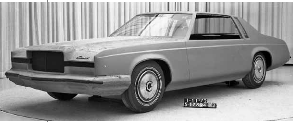
■ This full-sized, unfinished clay model of a larger Mark V shows an attempt to increase the size of the smaller Mark V, after it had been determined Wixom couldn't build a smaller Thunderbird and a smaller Mark V at the same time. The looks of the smaller Mark V did not transition well to a bigger car.
