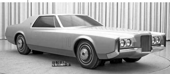
■ A little less than a year later, this 12-16-69 photo shows Ford designer Steve Sherer's proposed smaller Mark V, designed on a 114-inch wheelbase. The front has the classic Mark design cues, which the rest of the car lacks.
