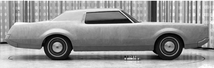
■ Left: This is the first photo found of a smaller Mark V proposal. It is dated 1-23-69. This car does not appear to have the same windshield slope as Marks traditionally have. According to retired Ford designer Dick Nesbitt, this car is almost identical in shape to the Torino/Montego-based Mark V in the Lincoln studio several years later. Center: From the back, the same car looks pinched. Designers identify this proposal as being on a 114-inch wheelbase. Right: From the front, this clay model of a smaller Mark V looks pinched. It was undoubtedly determined that the traditional Mark look didn't really carry through when the car was reduced in size.
