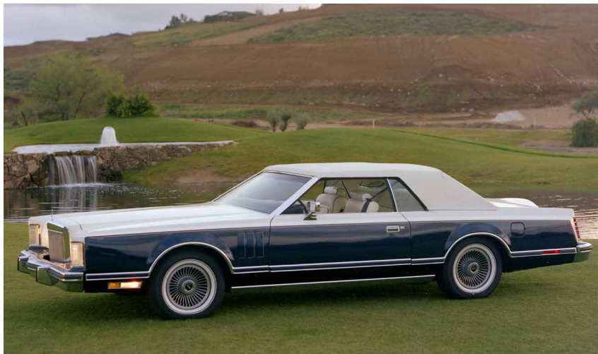
■ This 1979 Continental Mark V Bill Blass Edition was part of the popular Designer Edition models, tweaked with a canvas-covered (but not convertible) roof. The Mark V was 230 inches long that year, or 20 inches longer than the 1941 Continental. FORD MOTOR COMPANY, LINCOLN PHOTO ARCHIVE
