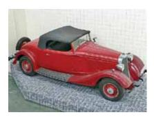
■ Dammann & Wagner tell us, in The Cars of Lincoln Mercury, that this 1933 Lincoln is Model 520-A with trunk deck. At a cost of \$2,900, it weighed about 4,750 lbs. and had a lined top. This was the first year for the new smaller V-12 engine of 381.7 cubic inches and 125 horsepower. The KA-1029 serial number was near the end of the run.
