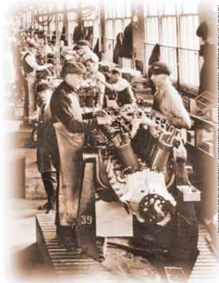
In the early days of the Lincoln plant, workers assemble the Liberty aircraft engine. The new museum will cover Lincoln history back to these earliest days.
